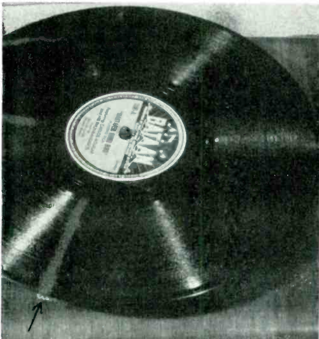
This disc, the folk song "Planting Rice" which I acquired in the Philippines has several scratches and a crack from the center hole to the edge. On the edge at the arrow you can see the tape which is applied to the bottom of the disc over the crack and the grease pencil mark which is rubbed into the surface of the crack. A scratch has been filled similarly at the upper left of the picture.
