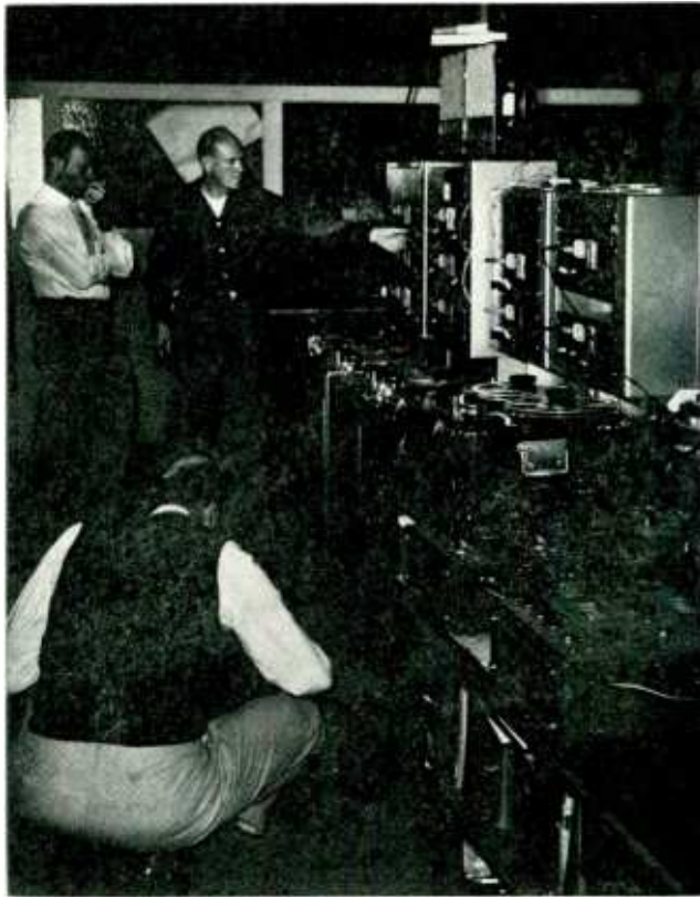
Equipment in the recording booth consisted of: (left to right) 1—full-track recorder (1/4" tape), 2—three-track stereo recorders (1/2" tape), 2—two-track stereo recorders (1/2" tape), 1—three-track stereo recorder (1/4" tape), and 2 more two-track stereo recorders (1/4" tape).
