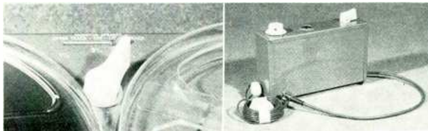
Left: the machine has three speeds, 7 \frac{1}{2} , 3 \frac{3}{4} and 1 \frac{7}{8} ips which are conveniently changed by turning the lever between the reels. Right: the external stereo recording amplifier contains volume, equalization controls and recording level indicator.
